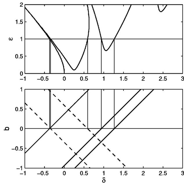
Fig. 5 Period one (continuous) and period two (dashed) boundary lines for Eq. (11) with  $\varepsilon = 1$ ,  $\kappa = 0.1$
