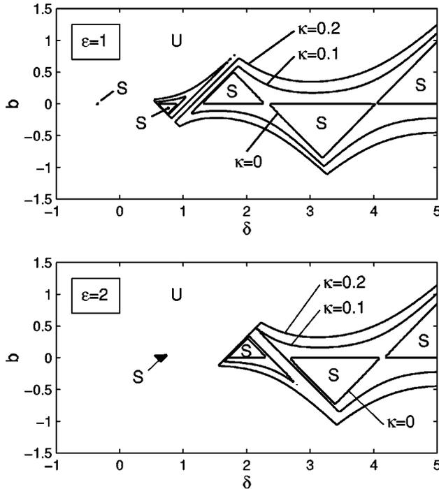
Fig. 7 Stability boundaries for the Eq. (11) obtained by the semi-discretization method
