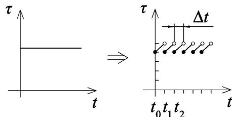
Fig. 6 Approximation of the time delay for  $m = 4$
