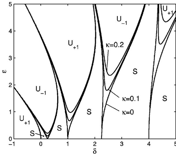
Fig. 1 Strutt-Ince stability chart of the damped Mathieu equation (4)
